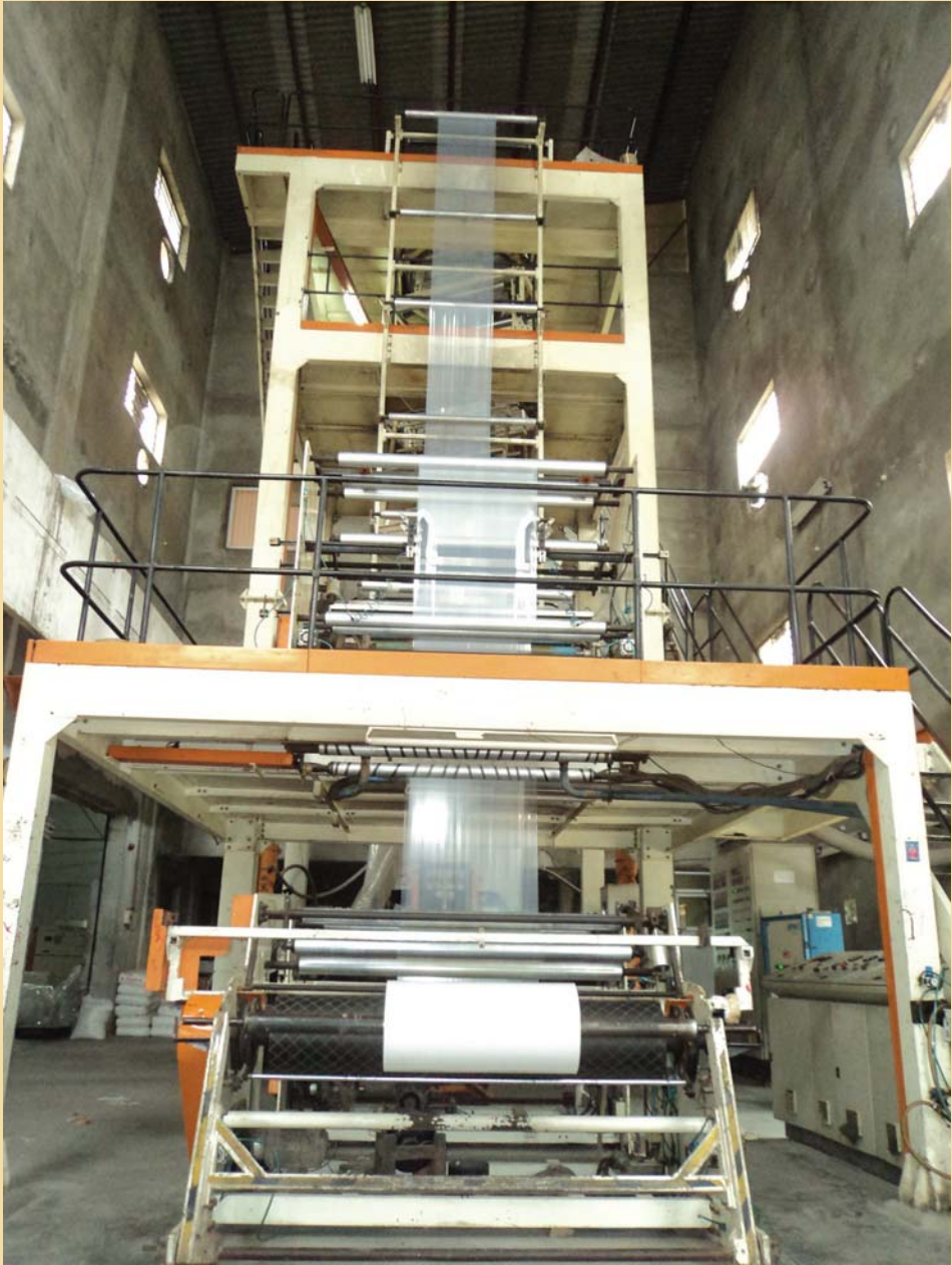
3 Layer Blown Film Plant
